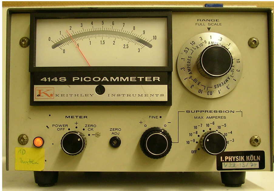
Figure 13: Photograph of the picoampere meter to measure the detector current
