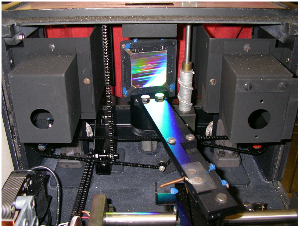
Figure 10: Photograph of the inside of the spectrometer. In the center of the picture, one sees the grating with the drive-mechanism in front. The two boxes in the far corners are the entrance slit and the output slit.
