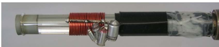
Figure 3: Sample head consisting of a tube filled with glycerol, which is surrounded by a copper coil and a capacitor forming a resonant circuit.
